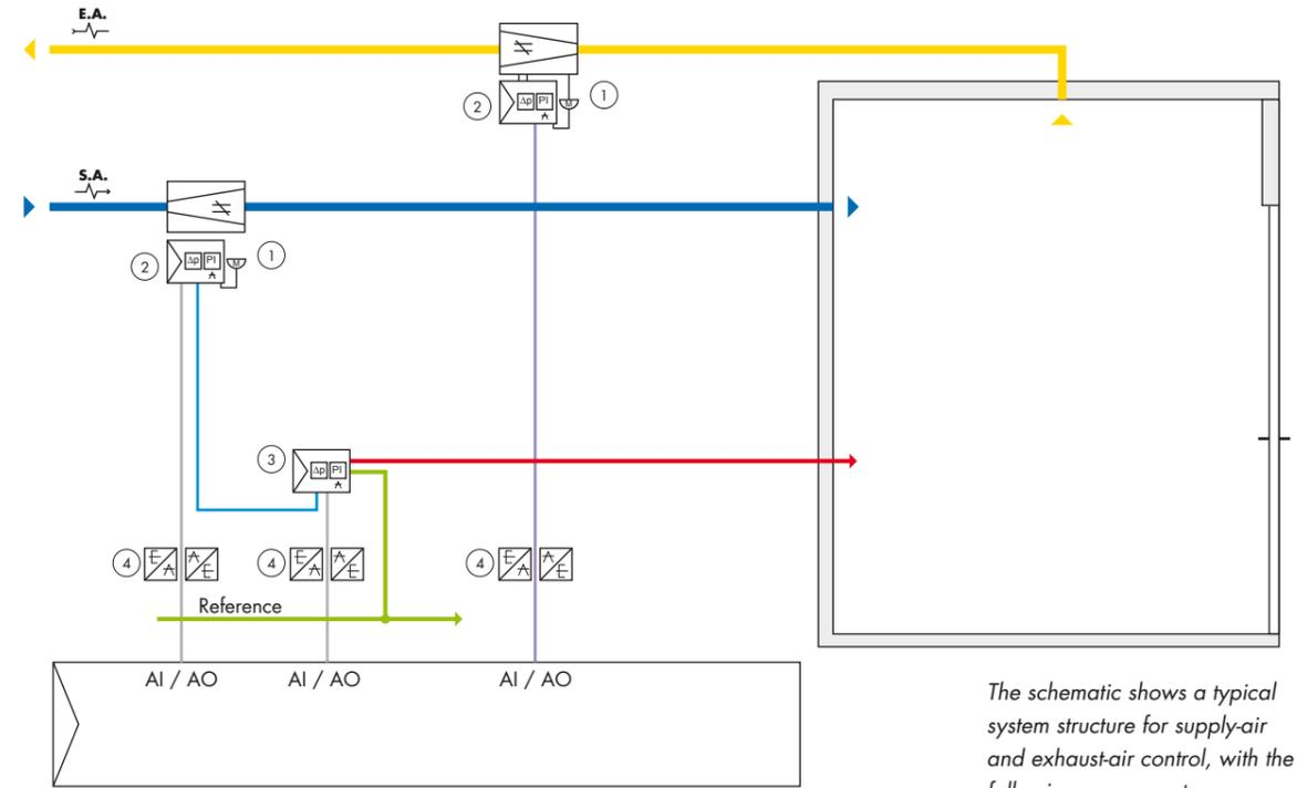
The schematic shows a typical system structure for supply-air and exhaust-air control, with the following components:-
