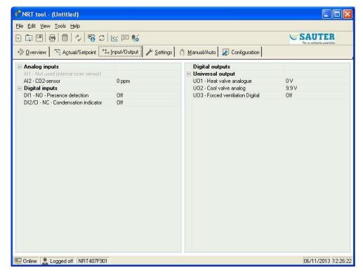
Shows actual values for all inputs and outputs. This is a read-only folder. No settings can be made here. Unconfigured inputs and outputs are grayed.
