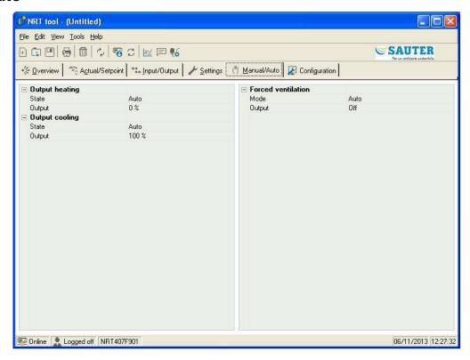
In this menu you can take manual command of most controller functions. It is very useful for testing purposes.
