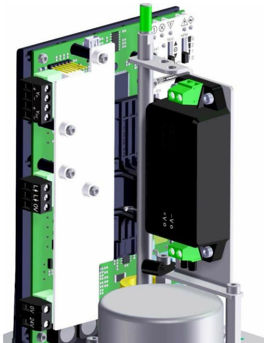
Fig. 12: Installation and connection of the power supply -Plus 2G 2,2 - 5 kN
