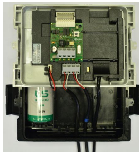
Picture 5.2 - Module installed in meter
