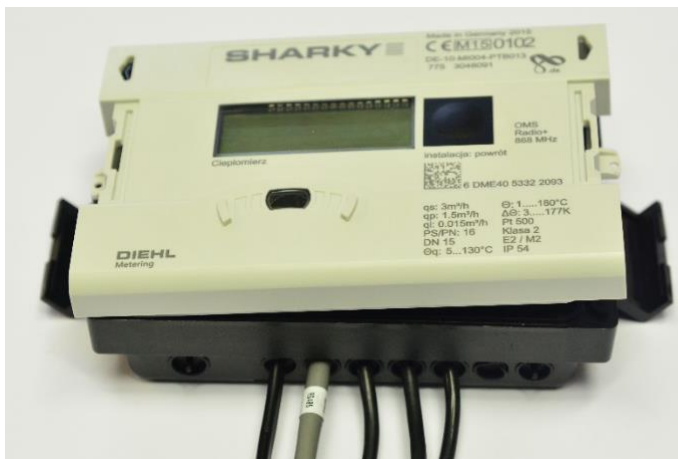
Picture 5.8 - Closing meter housing starting from left edge
